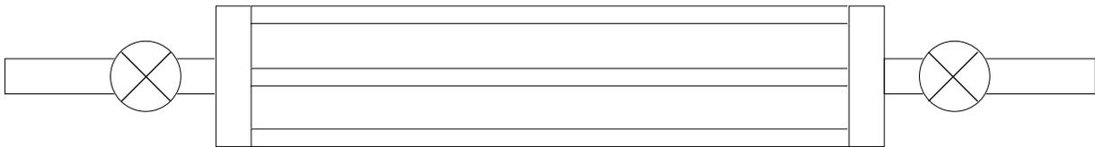
Figure2. Air sparger system with valves allowing control of air flow from end to end and air line to air line.
